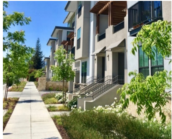
Fig. G.6: Access to ground floor residential units from the sidewalk using stoops.
