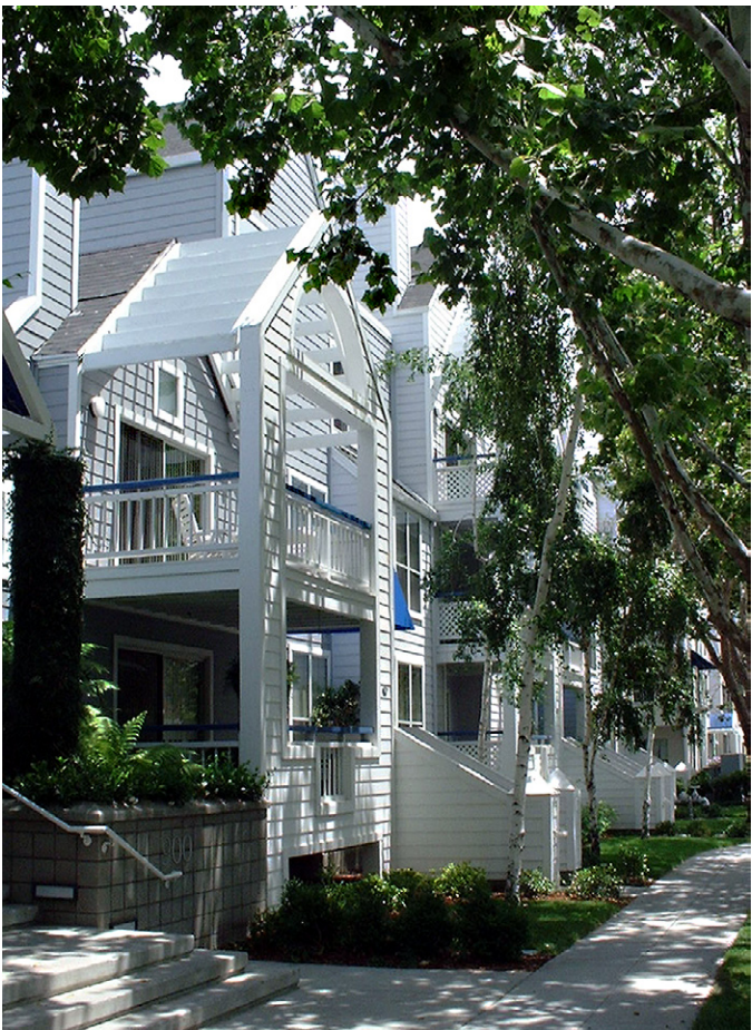
Primary building entries should be accessed directly from a publicly accessible street or walkway. All building entries should be clearly articulated with recesses, overhangs, special materials and/or detailing. Front doors should be substantial in appearance and one should be able to see through it.
