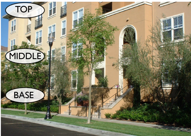
Building facades should have three recognizable design elements: a building base, middle and top. The base should visually support the building and may include thicker walls, special materials or darker colored materials.
