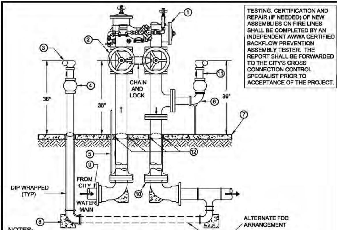
TESTING, CERTIFICATION AND REPAIR (IF NEEDED) OF NEW ASSEMBLIES ON FIRE LINES SHALL BE COMPLETED BY AN INDEPENDENT AWWA CERTIFIED BACKFLOW PREVENTION ASSEMBLY TESTER. THE REPORT SHALL BE FORWARDED TO THE CITY'S CROSS CONNECTION CONTROL SPECIALIST PRIOR TO ACCEPTANCE OF THE PROJECT.
