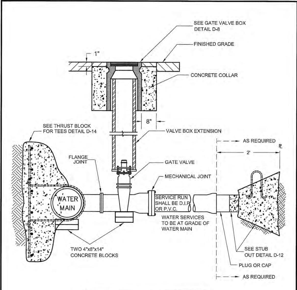
GATE VALVE ANCHOR REQUIRED WHEN VALVE IS NOT CONNECTED BY FLANGE JOINT TO MAIN TEE
