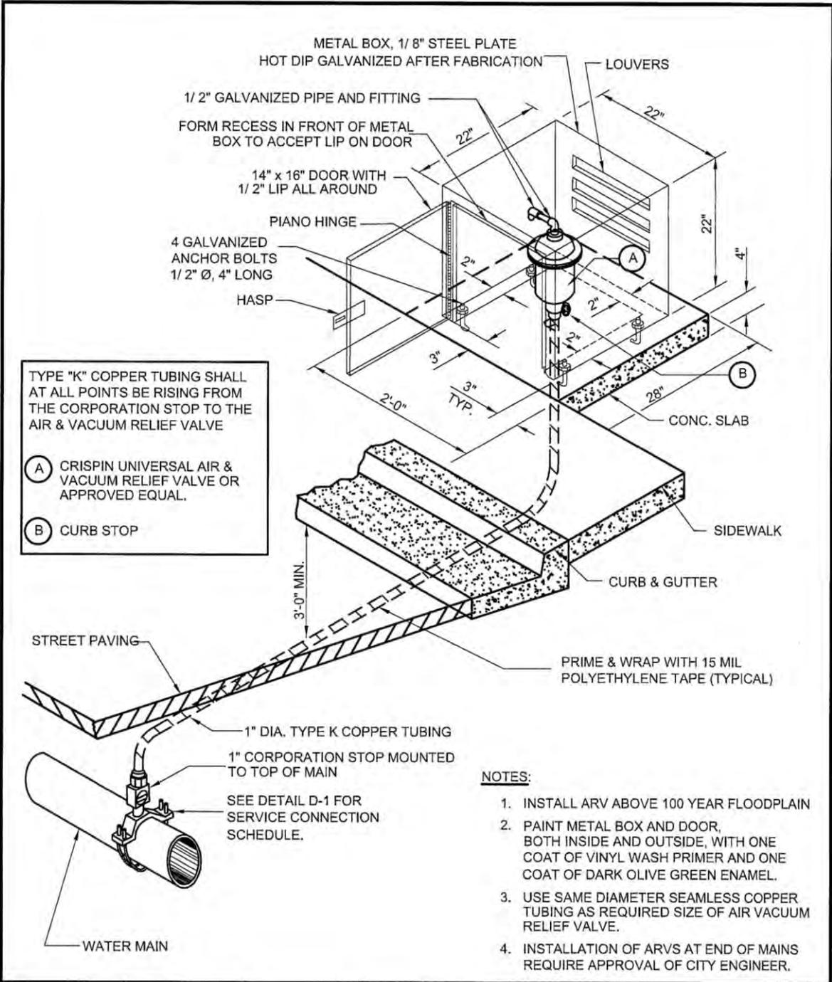
TYPE "K" COPPER TUBING SHALL AT ALL POINTS BE RISING FROM THE CORPORATION STOP TO THE AIR & VACUUM RELIEF VALVE
