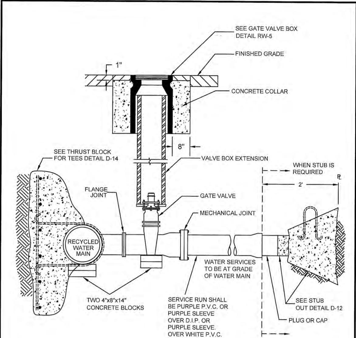
GATE VALVE ANCHOR REQUIRED WHEN VALVE IS NOT CONNECTED BY FLANGE JOINT TO MAIN TEE
